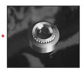
CKF2 and CKFS2 broaching-type fasteners are designed for use on printed circuit boards and on most brittle or hard materials; such as, glass laminates, epoxy or resin with paper, nylon, or canvas bases. They are also used on materials too thin or unsuitable for threading, such as acrylic and polycarbonate panels.
